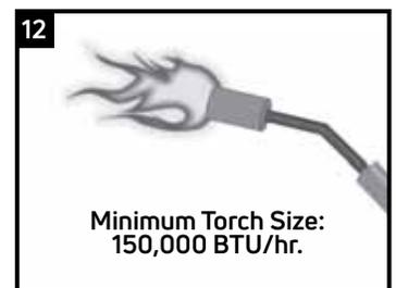
Use moderate flame intensity for sleeve shrinking. Remove protective heat shields prior to next step.
