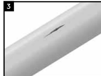
Deep PE jacket gouges not penetrating through to foam
