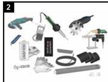
Hot Air Tool, Field Extrusion Welder, Welding Clamp, Polyethylene Welding Material (PE Rod), Knife, Chamfering Tools, Surface Preparation Tools (sandpaper, solvent, rags), Thermometer, Triangle Scraper, Angle Grinder with 40-60 Flap Disks, PPE.
