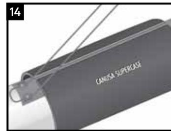
CSC-XP-R is wrapped around the pipe and fixed in a clamp tool in order to hold it properly for hot air and extrusion welding.
