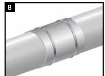
Prepared cavity, which does not encompass the entire circumference of the pipe, is foamed using a removable steel mould. Suitable foam shall be used.
