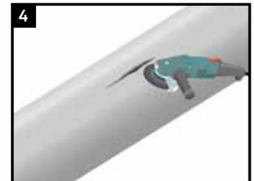
Remove all protruding PE material and expose fresh PE material in preparation for PE welding along and around the entire gouge. Clean the affected area with suitable solvent.
