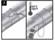
Pre-heat the joint area (steel and adjacent mainline coating) to minimum 90°C (195°F) with the appropriate propane torch. Using a temperature measuring device, ensure that the correct temperature is reached on the steel and at least 50 mm (2") on each side of the sleeve width. Do not use an intense flame on the mainline coating.
