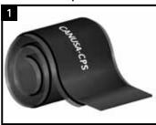
GTS-65-EN Global Transmission Sleeves are shipped pre-cut with a pre-attached closure. Bulk quantities are also available. When supplied in bulk refer to GTS-80-ISO Sleeve Cutting Guidelines for recommended closure dimension, sleeve cut lengths and corner cuts (15 mm x 50 mm - 0.6" x 2"). The sleeve adhesive is protected from contamination by an inner liner.
