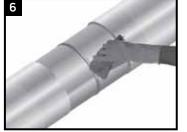
Wipe clean or air blast the steel and coated areas to remove foreign materials.
