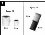
Follow the Preparation, Mixing and Application instructions provided with the supplied Canusa Epoxy Type E-WF Pack. For bulk quantities: mix the primer cure with the primer base 3 parts base to 1 part cure by volume). Stir for a minimum of 1 minute to assure uniform mixture.
