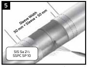
Warm the joint area to  $40-50^{\circ}$ C ( $100-120^{\circ}$ F) before grit blasting. Thoroughly clean the weld area with a blaster to "near white metal" SIS Sa 21/2 or equivalent. Abrade or sweep blast the mainline coating adjacent to the weld area to a distance 50 mm (2") beyond the sleeve width.
