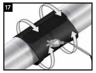
Continue heating from the centre toward one end of the sleeve until recovery is complete. In a similar manner, heat and shrink the remaining side.
