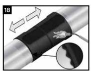
Shrinking has been completed when the adhesive begins to ooze at the sleeve edges all around the circumference. Finish shrinking the sleeve with long horizontal strokes over the entire surface to ensure a uniform bond.
