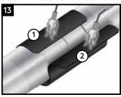
Wrap the sleeve loosely around the pipe, ensuring the appropriate overlap. Gently heat the backing of the underlap and the adhesive side of the overlap.
