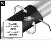
Using the appropriate sized torch, begin at the centre of the sleeve and heat circumferentially around the pipe. Use broad strokes. If utilizing two torches, operators should work on opposite sides of pipe.
