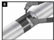
Apply mixed Epoxy to a minimum uniform thickness of 6 mils on all exposed bare metal plus 10 mm (0.5") onto the adjacent pipe coating using the applicator pads as supplied or an approved tool.
