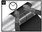
Centre the sleeve over the joint so that the sleeve overlaps between the 10 and 2 o'clock positions. Press the underlap firmly into place.
