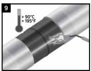
Using an appropriately sized induction coil or propane torch(es), pre-heat the joint area (epoxy and parent coating) to a minimum of 90°C (195°F) until primer reaches a dry-to-touch state. Abraded parent coating must be reheated to a min. 90°C (195°F) if its temperature dropped during force curing of the epoxy. Do not use an intense flame on the mainline coating. If a film develops on the mainline coating because of excessive preheat, use a surface abrasion tool to remove it.
