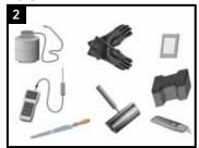
Propane tank, hose, torch & regulator; Appropriate tools for surface abrasion; Epoxy application accessories & wet film thickness gauge; Knife, roller, rags & Canusa approved solvent cleanser; Digital thermometer with suitable probe; Standard safety equipment: gloves, goggles, hard hat etr
