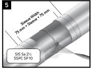
Warm the joint area to 40-50°C (100-120°F) before grit blasting. Thoroughly clean the weld area with a grit blaster to "near white metal" SIS Sa 2½ or equivalent. Abrade or sweep blast the mainline coating adjacent to the weld area to a distance 75 mm (3") beyond the sleeve width
