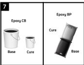
Follow the Preparation, Mixing and Application instructions provided with the supplied Canusa Epoxy Type E-WF. For bulk quantities: mix the primer cure with the primer base (3 parts base to 1 part cure by volume). Stir for a minimum of 1 minute to assure uniform mixture.
