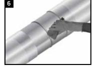
Using a dry, grease- and lint-free cloth, wipe clean or air blast the steel and coated areas to remove foreign materials.
