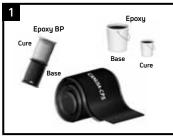
GTS-80-ISO Global Transmission Sleeves are shipped pre-cut with a pre-attached or separate closure. Bulk quantities are also available. When supplied in bulk refer to GTS-80-ISO Sleeve Cutting Guidelines for recommended closure dimension, sleeve cut lengths and corner cuts (15 mm x 50 mm - 0.6" x 2"). The complete joint system also uses a liquid epoxy.
