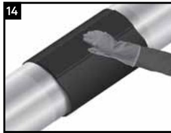
With the green-yellow coloured adhesive side facing down, firmly press the entire closure seal into place. Ensure that the closure is centred evenly over the underlap-overlap sleeve seam. If necessary, add additional heat to the closure underside in cold conditions, using a low flame intensity.
