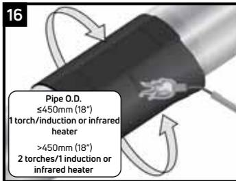
Using the appropriate sized torch, begin at the centre of the sleeve and heat circumferentially around the pipe. Use broad strokes. If utilizing two torches, operators should work on opposite sides of pipe.
