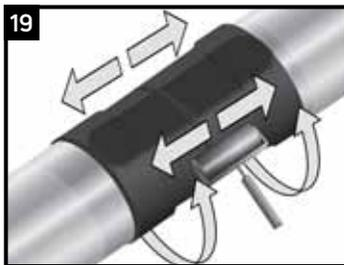
While the sleeve is still hot and soft, use a hand roller to gently roll the sleeve surface and push any trapped air up and out of the sleeve, as shown above. Continue the procedure by also firmly rolling the closure with long horizontal strokes from the weld outwards.
