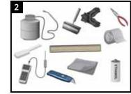
Propane tank, hose, torch & regulator; Wire brush, sand paper, triangular scraper; Knife, rags & appropriate solvent (e.g. Ethanol or Isopropyl alcohol); Temperature measuring device, ruler, pencil, Standard safety equipment; gloves, goggles, hard hat, etc.
