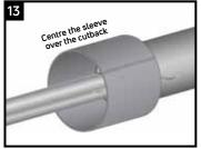
Centre the CanusaTube<sup>™</sup> PLX over the sealing area. Ensure the PLX will overlap the jacket and service pipes by at least 50 mm. Ensure the edge of the PLX lines up with the markings on the jacket pipe.
