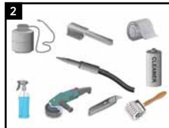
Appropriate tools for surface abrasion and preparation (wire brush/power wire brush or grit blaster, abrasive paper (40-80 grit), Knife, lint free rags, approved solvent and water spray bottle. Standard safety equipment: gloves, safety glasses, hard hat, etc.
