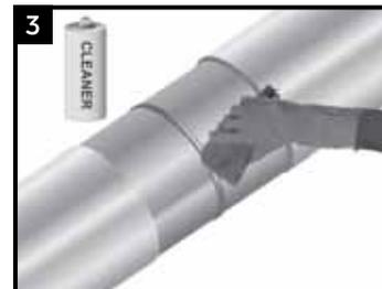
Clean exposed steel and adjacent pipe coating with an approved solvent (Acetone, MEK, Alcohol >96%) to remove the presence of oil, grease, and other contaminants if present. Ensure that the pipe is dry prior to mechanical cleaning.
