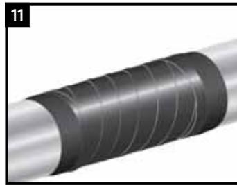
Allow the Scar-Guard<sup>®</sup> XL to reach a Shore D Hardness of 70 prior to pulling. Scar-Guard<sup>®</sup> XL is fully cured at a Shore D Hardness of 83 @ 72°F.
