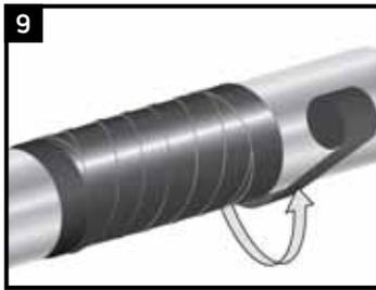
Apply compression film in the same direction as the previous layers with a 50% overlap. Start min. 50mm (2") beyond the outer edge of the Scar-Guard<sup>®</sup> XL, pulling firmly during application.
