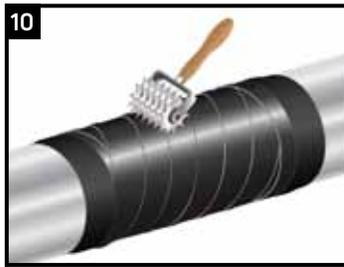
Perforate the compression film using a wire brush (or other perforating device) by tapping firmly on the tape with the metal bristles. Perforation allows the CO<sub>2</sub> gas generated by the curing process to escape. Compression film may be removed after material hardens and either discarded or left in place.
