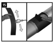
Bulk sleeve roll with separate closure: Heat the adhesive side of the closure to activate the adhesive before centering the closure over the overlap and pressing it firmly down into place.
