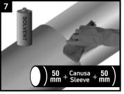
De-grease the surface (width of sleeve + 50 mm on each side) using a grease and lint-free rag soaked in ethanol (min. 94%) or other suitable solvent.
