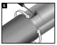
Clean the edges of the casing to remove any sharp corners and burrs, foam and dirt, using a triangular scraper.
