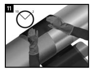
Centre the sleeve over the area to be sealed, so that the sleeve overlaps between the 10 and 2 o'clock positions. Press the underlap firmly into place.
