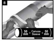
Roughen the surface (width of sleeve + 50 mm on each side) using 40-60 grade sandpaper.
