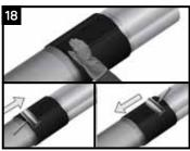
As the sleeve is being shrunk, the closure shall be occasionally patted down with a gloved hand or rolled to ensure that it is well bonded to the sleeve and it is not lifting anywhere.
