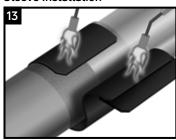
Wrap the sleeve loosely around the pipe, ensuring the appropriate overlap. Gently heat the backing of the underlap and then gently heat the adhesive side of the overlap.
