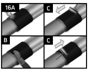
Heat the closure with a moderate flame intensity and pat it down with a gloved hand or a roller across its entire length. Make sure that the closure is firmly attached to the underlying sleeve and it is not lifting anywhere. Smooth any wrinkles by gently working them outward from the center of the closure with a roller or by patting the closure down.
