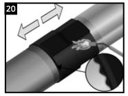
Shrinking has been completed when the adhesive begins to ooze at the sleeve edges all around the circumference. Make sure the edges of the sleeve are not lifting anywhere around the circumference of the pipe. Finish shrinking the sleeve with long horizontal strokes over the entire surface to ensure a uniform bond.
