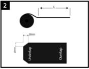
Cut the required length (L) of sleeve material from the bulk roll.
