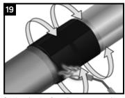
Continue heating from the centre toward one end of the sleeve until recovery is complete. In a similar manner, heat and shrink the remaining side. At the same time continue to pat down or roll the closure to ensure its conformity to the sleeve along its entire width.
