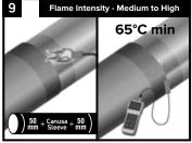
Using medium to high intensity flame, pre-heat and activate the surface to be covered with heat shrink sleeve and min 50 mm on each side of the sleeve to a minimum temperature of 65°C. The flame shall be kept perpendicular to the surface of the pipe and casing during pre-heating. Check the temperature around entire circumference of the pipe with a touch probe.
