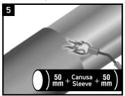
Dry the surface of the casing and jacket pipe (width of sleeve + 50 mm on each side) with moderate flame intensity. Clean the surface with a dry, grease and lint-free rag to remove any grease or dirt.
