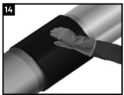
Pre-cut sleeves with pre-attached closure: Heat the adhesive side of the closure to activate the adhesive before pressing it firmly into place.
