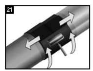
While the sleeve is still hot and soft, use a hand roller to gently roll the sleeve surface and push any trapped air up and out of the sleeve, as shown above. If necessary, reheat to roll out air. At the same time, the closure shall also be patted down with a gloved hand or rolled to ensure its full conformance to the underlying sleeve.
